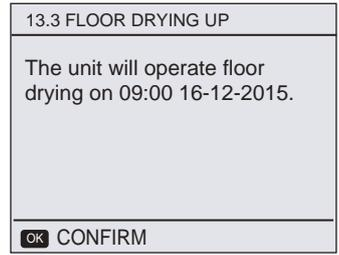
When the cursor is on OPERATE FLOOR DRYING? Use ◀ ▶ to scroll to YES and press OK. The page will be displayed as follows:
