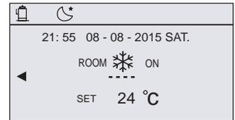
If you set WATER FLOW TEMP. to NON, and set ROOM TEMP. to YES, then the room temperature will be displayed on the home page, and the room temperature will work as the target temperature. The target outlet water temperature can be calculated from the climate related curves.
